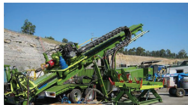
MAXIBOR'S GALLAGHER HDD660E ELECTRIC MAXI-RIG.
